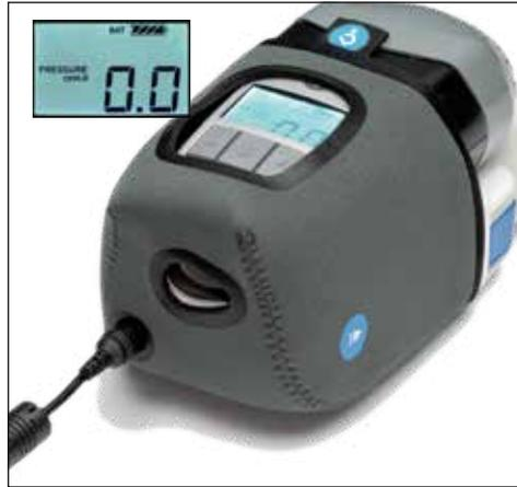
The Z1 can be removed from the PowerShell by pressing the two (▶) icons on the sides of the PowerShell and sliding the Z1 out. The battery can be removed from the PowerShell by the two blue buttons on the battery shuttle and sliding the battery out.
