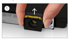
With the device on a stable level surface, grip the retention clip on the back of the device and pull up to open.
