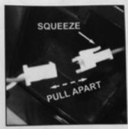
Connect the adapter base by joining its connector to the main unit connector. Push together and snap into place. Note: at this point you should make sure that the switch on the underside of your main unit is in the ON position.
