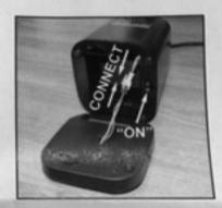
Attach the base to the main unit by inserting the long rear tab into its matching slot on the main unit. Then pivot the front of the base so that it comes together with the main unit and the front tab clicks into place.
