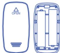
Figure 3. Batteries Installation
