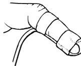
**Figure XI: Flex Sensor with tape strain relief.**
