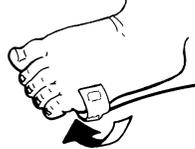
**Figure XIII: Neonatal Flex Sensor on foot.**
