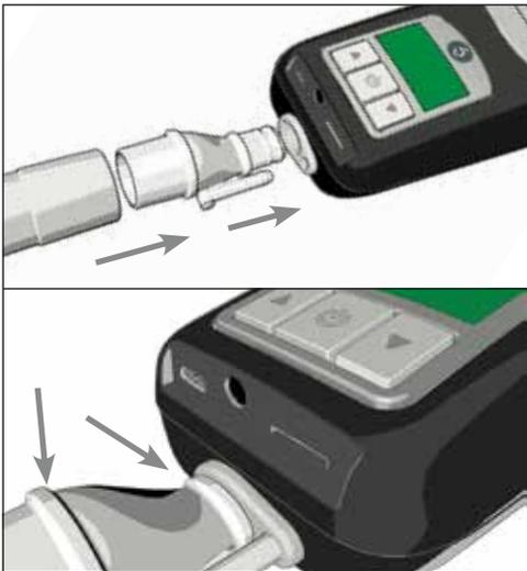
**2.** Plug the power supply (AC to DC power adapter) into the Z1 as shown and into a wall outlet. The Z1 will power up in standby mode. The display will read 0.0. The Z1 display will always be active whenever the device is receiving power.
