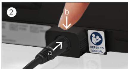
(a) Plug the power connector into the device power inlet then (b) push down the retention clip to secure in place.
