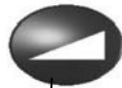
Manual ramp on or off when the blower is on; in Standby mode it is used to review Patient Settings
